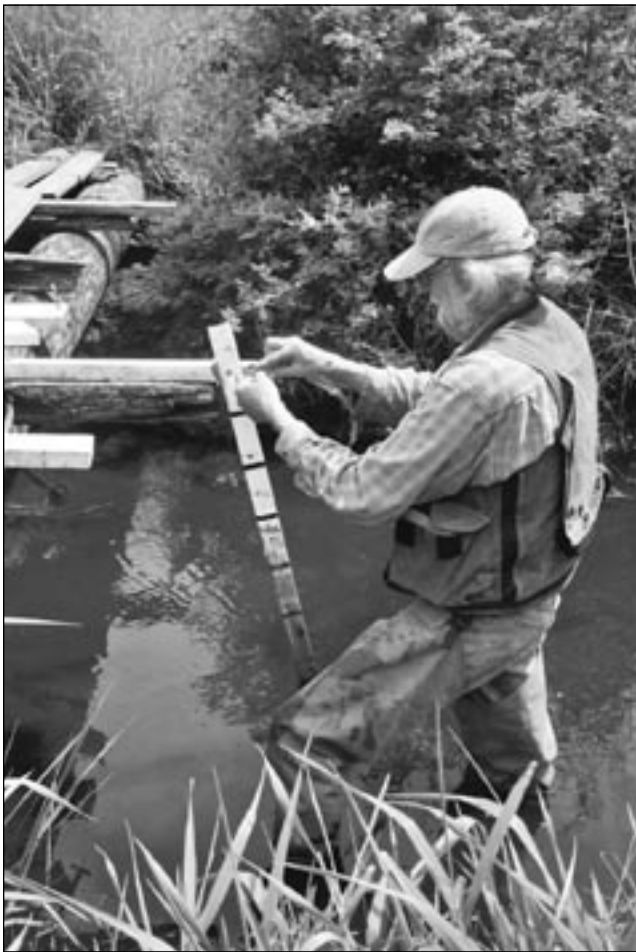
David Crabb, WT Field Technician, installing a temperature data logger in Maxwellton Creek.
