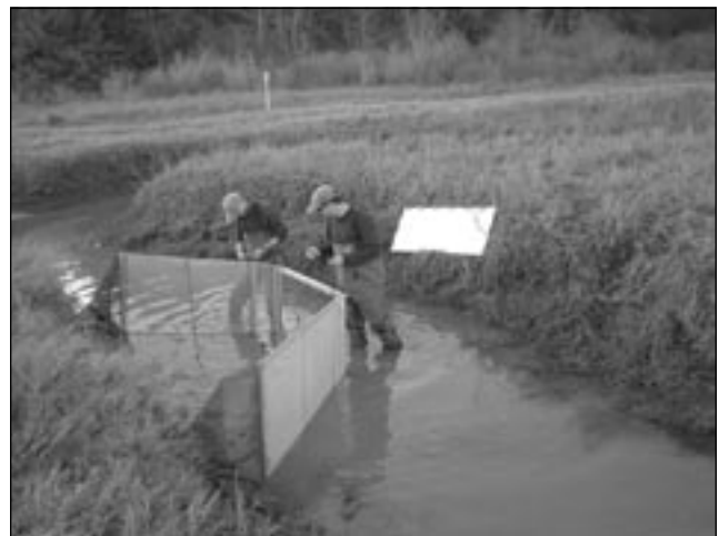
WT Executive Director Kurt Beardslee and WT Conservation Biologist Micah Wait setting up a prototype videographic fish weir in a blind tidal channel on the Dosewallips estuary.
