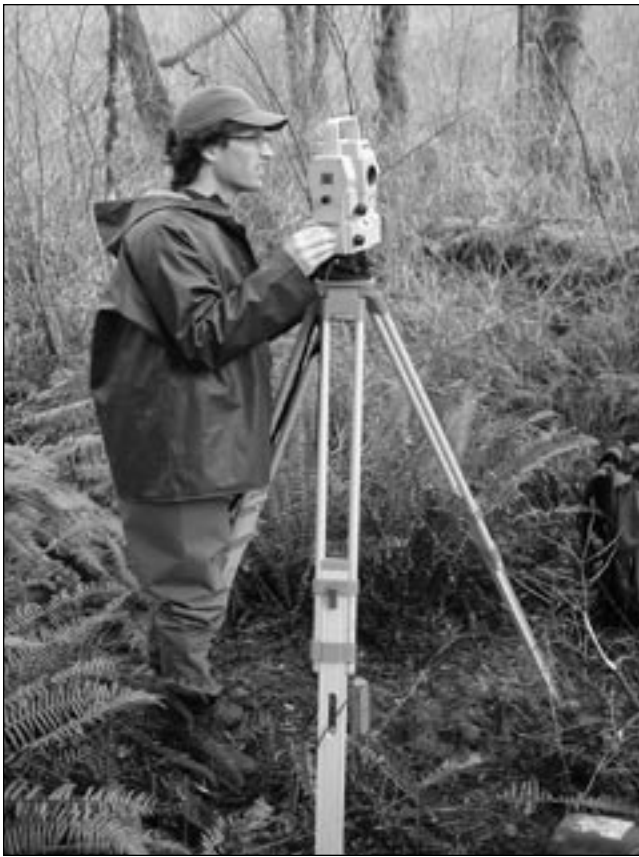
Joseph Yacker, WT GIS Specialist, using the Total Station to survey and record elevation data in an area of dense vegetation.
