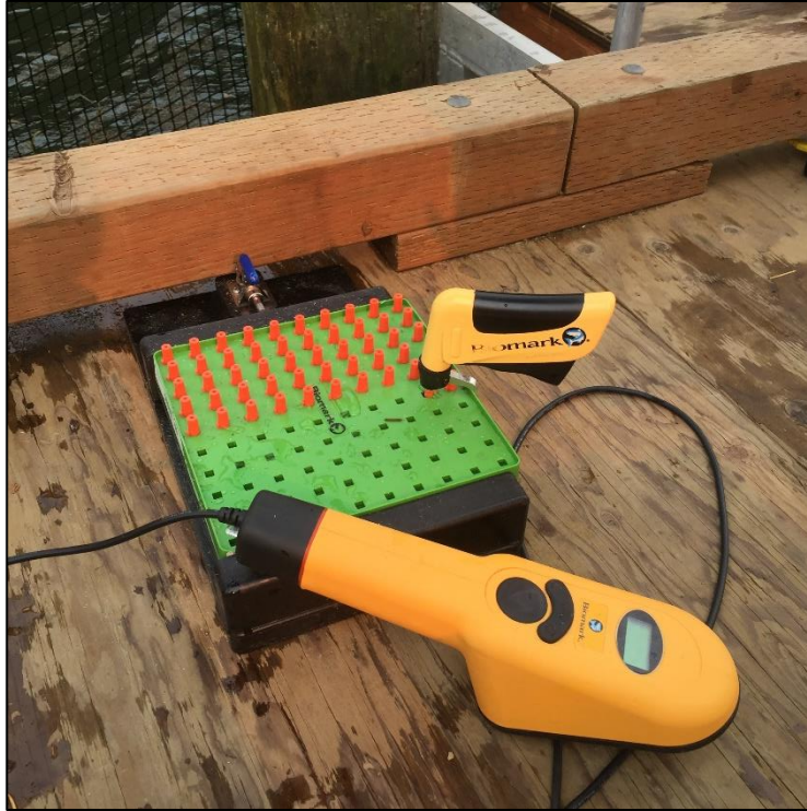
Figure 2-7. Biomark 601 reader, MK-25 Rapid Implant Gun, and 12.5 mm 134.2 kHz full duplex PIT tags used for the mark-recapture study. Photo by Adrian Tuohy (WFC 2018).
