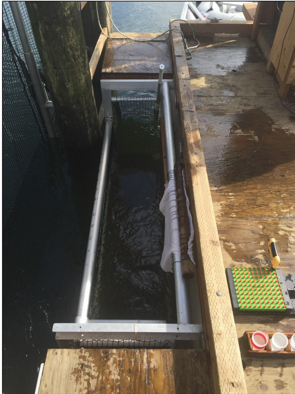
Figure A-8. The perforated live-well compartment positioned adjacent to the spiller. This compartment enabled river flows to continuously oxygenate the water for recovering fish. The live well door can be viewed near the top of the photo. Photo by Adrian Tuohy (WFC 2018).
