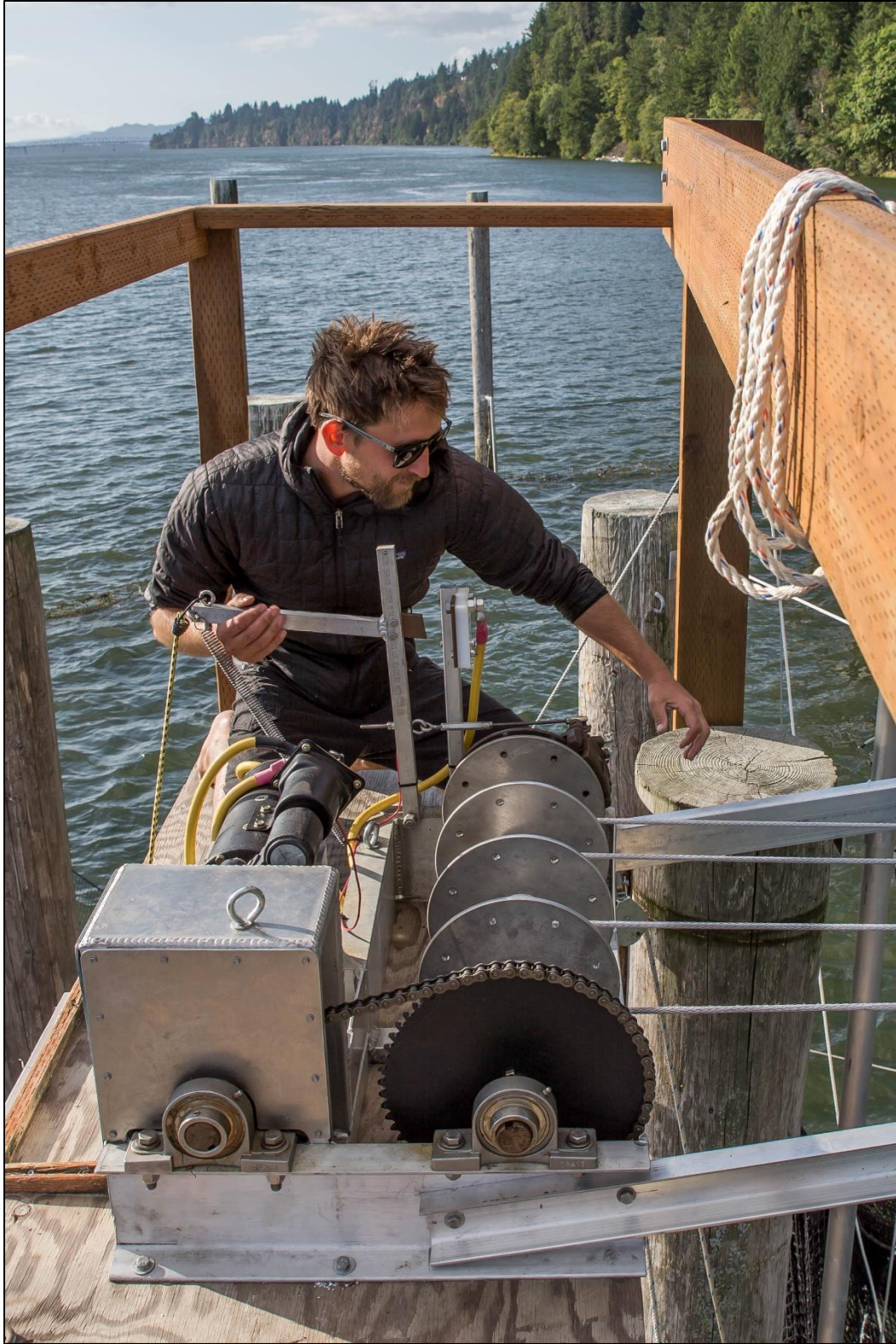
Figure A-11. WFC field staff lift the spiller compartment with a solar powered electric winch. Photo by Jamie Glasgow (WFC 2018).
