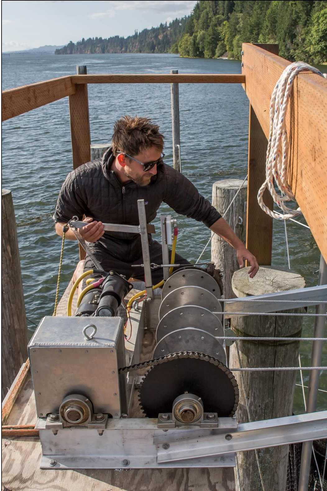
Figure D-17. WFC field staff lift the spiller compartment with a solar powered winch in 2017.
