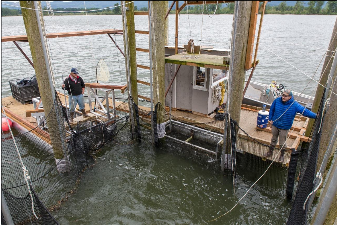
Figure D-28. WFC staff fishing the passive spiller trap design in May 2019.
