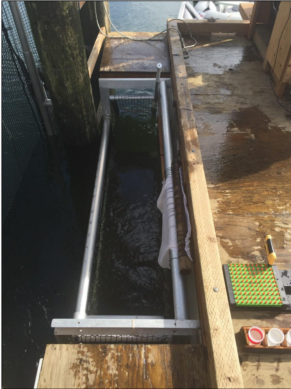
Figure D-12. The perforated live-well compartment positioned adjacent to the spiller. This compartment enabled river flows to continuously oxygenate the water for recovering fish. The live well release door can be viewed near the top of the photo.
