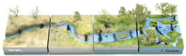
Reach-scale restoration over time, using beaver dam analogs.
