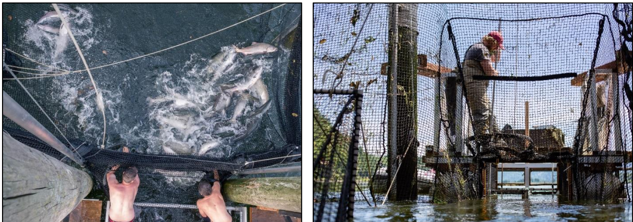
Figure V-4. The prototype spilling technique (left) used line-and-pulley and an electric winch to brail groups of captured fish to a live well for sorting. The modified passive design (right) employed an upstream tunnel from the spiller compartment to allow individual fish to migrate at their own volition from the spiller to an attached upstream live well for sorting and passive release with zero air exposure, handling, and brailing.
