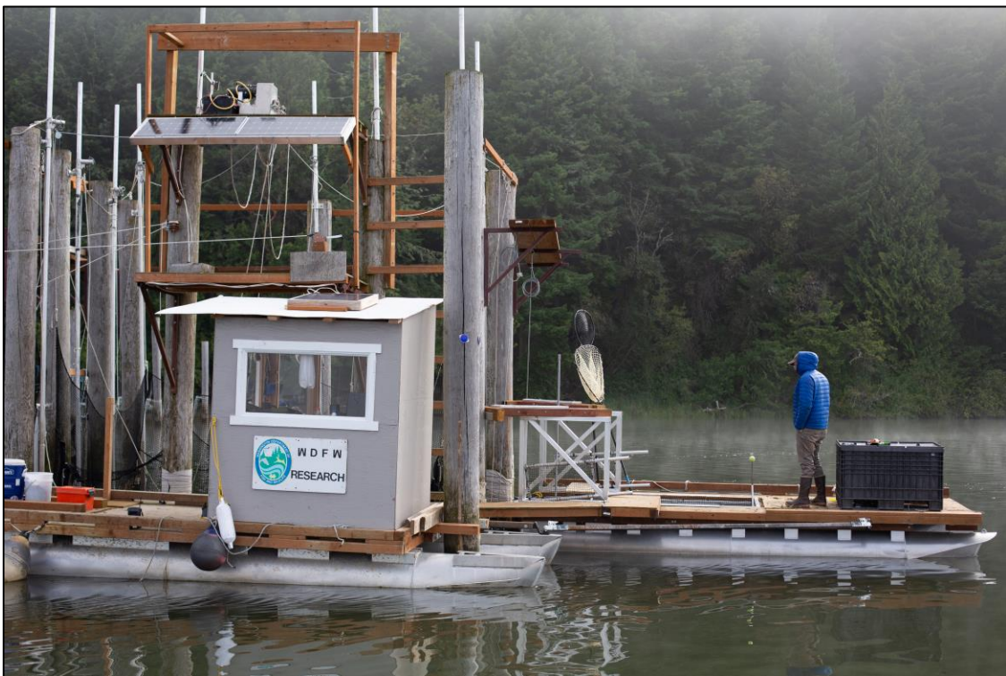
Figure D-31. The new upstream live-well dock (featured on the right) which enabled the passive spiller method in 2019, and the old live-well dock and modified data booth (left) where the winch-and-spill treatment operated.
