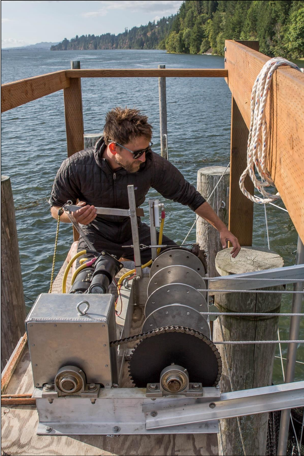
Figure D-17. WFC field staff lift the spill compartment with a solar powered winch in 2017.
